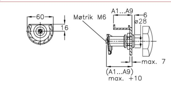
Door + frame thickness = 27-35 Measure type = A3
